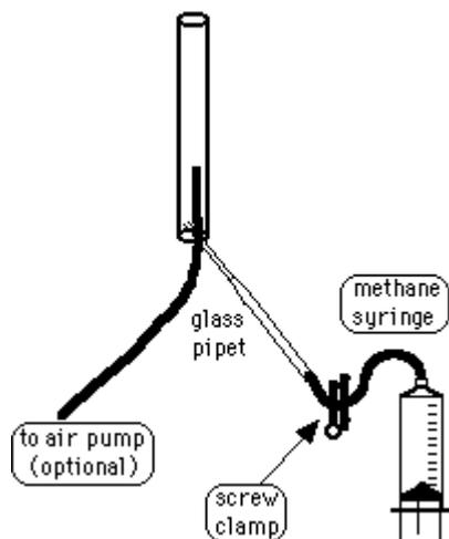
Figure 4. A glass tube Bunsen burner
