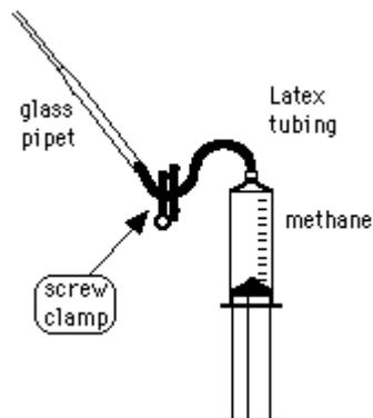
Figure 3. Screw clamp controls gas flow rate.
