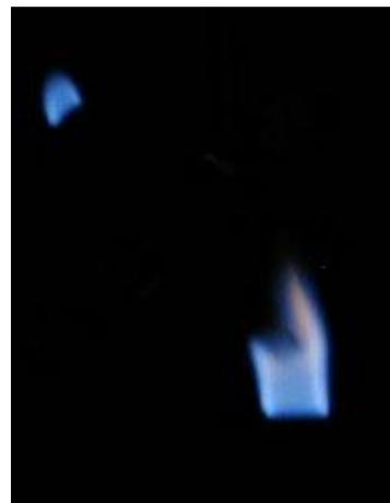
**Washing gas with water removes sodium and methane burns blue**
